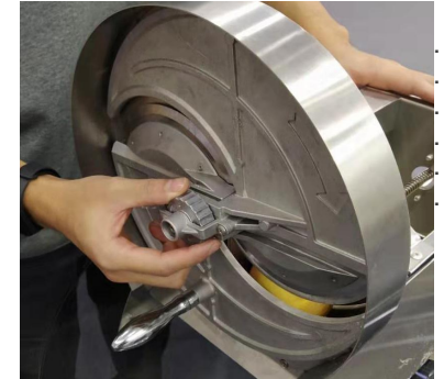
2.Clockwise can adjust it thinner Counterclockwise will be thicker
